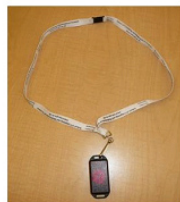
IR Tag with lanyard (worn by PAX & logs ID for each beacon it sees)
