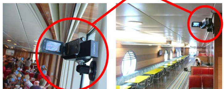
Video cameras positioned to view passenger seating areas
